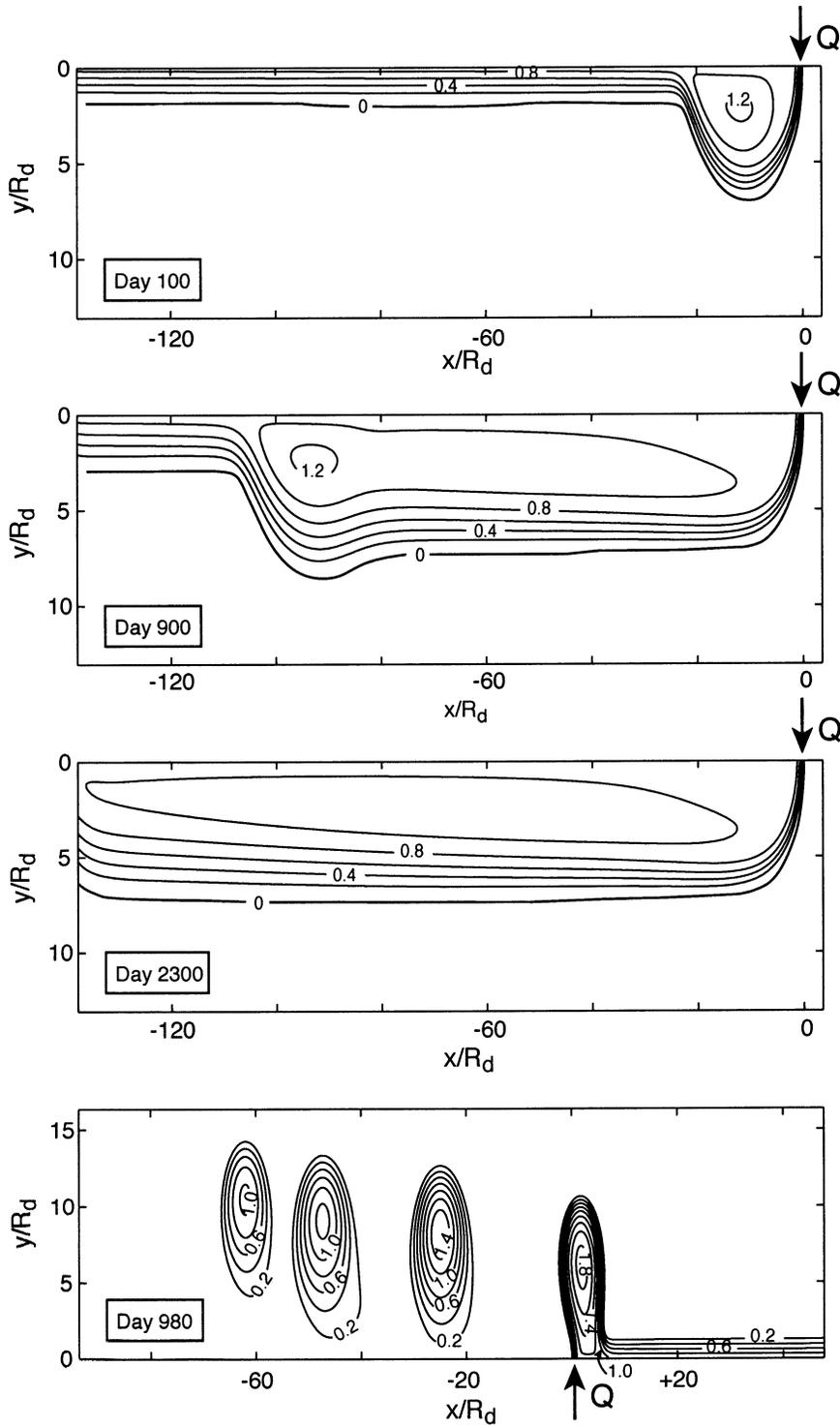
FIG. 7. Same as the zero potential vorticity case (Fig. 6) except that the outflow's potential vorticity is now finite ( $H_p = 1100$  m;  $H = 470$  m). It shows that the difference between the two is minimal.
