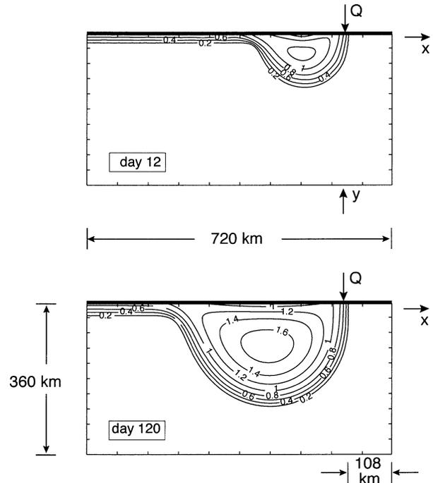
FIG. 4. Nondimensional  $f$ -plane thickness contours ( $h/H$ ) for a zero PV outflow. Note that the gyre is growing in time. Physical constants:  $f = 10^{-4} \text{ s}^{-1}$ ;  $g' = 2 \times 10^{-2} \text{ m s}^{-2}$ ;  $Q = 20 \text{ Sv}$ ;  $R_d = 30 \text{ km}$ ;  $H = 450 \text{ m}$ ; grid size  $\Delta x = \Delta y = 3.6 \text{ km}$ ; time step,  $\Delta t = 5 \text{ min}$ ; eddy viscosity,  $360 \text{ m}^2 \text{ s}^{-1}$ . Adapted from Nof and Pichevin (2001).
